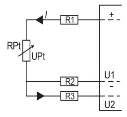
The resistance of all the connection wires must be identical, i.e.  $R_1 = R_2 = R_3$ . In the Table below, there are shown examples of errors caused by the resistance difference of 0.1  $\Omega$  and of 1.0  $\Omega$  between the wires of a 3-wire connection line for Pt 100 and Pt 1000.
