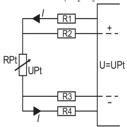
This connection line is used when a vary hugh accuracy of temperature measuraments is required. In the case of a 4-wire connection line, the impact of resistor's wires resistance is totally eliminated. For practical reasons, the resistance of a single wire input circuit of RTD should not be higher than 11  $\Omega$ .
