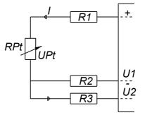
The resistance of all the connection wires must be identical, i.e.  $R_1=R_2=R_3$ . In the Table below, there are shown examples of errors caused by the resistance difference of  $0.1\Omega$  and of 1.0  $\Omega$  between the wires of a 3-wire connection line for Pt 100 and Pt 1000.
