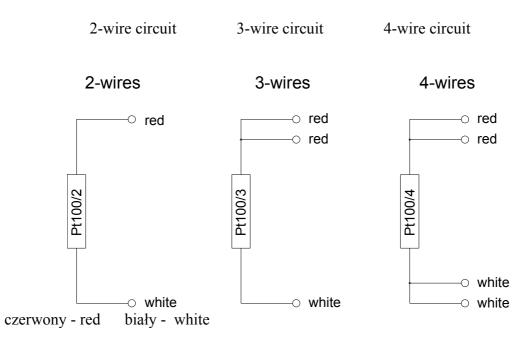
Two Measurement Circuits
