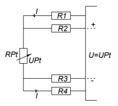
This connection line is used when a very high accuracy of temperature measurements is required. In the case of a 4-wire connection line, the impact of resistor's wires resistance is totally eliminated.
