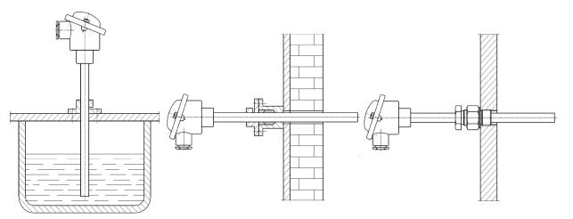
Examples of sensors assembly in the pipeline:
