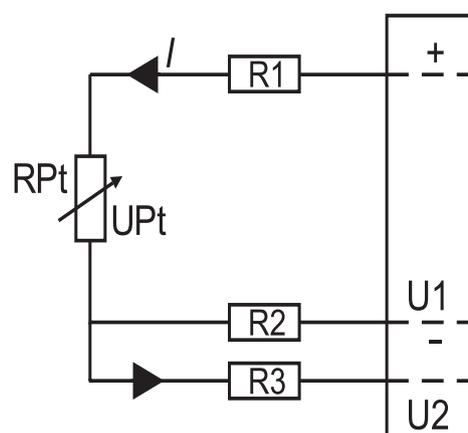
The resistance of all the connection wires must be identical, i.e.  $R_1=R_2=R_3$ . In the Table below, there are shown examples of errors caused by the resistance difference of 0.1 Ω and of 1.0 Ω between the wires of a 3-wire connection line for Pt100 and Pt1000.
