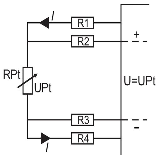
For practical reasons, the resistance of a single wire input circuit of RTD should not be higher than 11  $\Omega$ .
