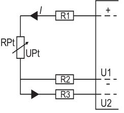
Connecting wires must have identical resistance  $R_1 = R_2 = R_3$ . The table below provides examples of errors for 3-wire connection for Pt100 and Pt1000 for difeference of wire resistance 0.1 $\Omega$  and 1 $\Omega$ .
