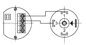
Single sensors without transmitters can be mounted with peripheral devices with the use of 2-, 3- or 4-wire configuration – details are provided below; double sensors: only 2-wire configuration; similarly sensors with transmitter (only single):
